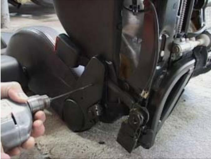
Time to separate the back and the bottom: just the two frames will be separated; the wires will remain connected.
