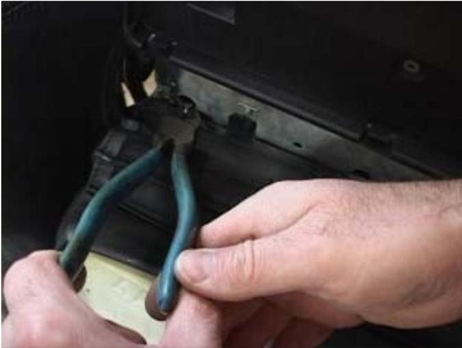
So now the cushion and leather are free of the base. If you are also replacing the side bolster, remove the hog rings and replace it now.
