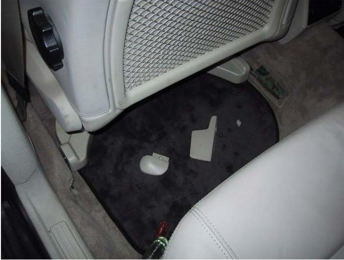
The front bolts are trimmed with two plastic covers. To remove the covers, press down and slide them toward the front of the car.
