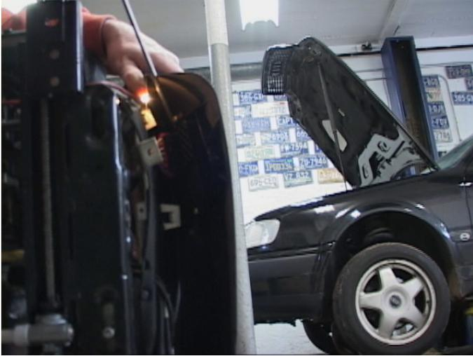
The black plastic trim on the inner side is clipped into three holes, then a plastic plug is inserted into each hole to keep the fit tight. To remove the trim, the plugs must be removed. Two are easily pushed through with a small screwdriver; the third is not so easy. It can be pushed almost all the way through, but still may not go. I drilled a small hole in it, inserted a drywall screw and pulled it out. Failing this, just force it through. Pop the trim off.
